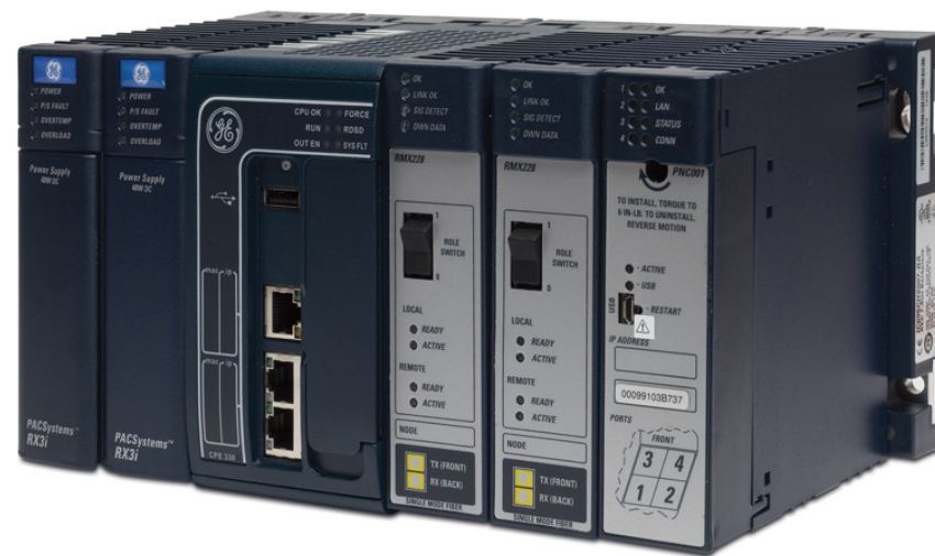
The “brain” of the system is a PACSystems Rx3i in redundant configuration, which interfaces with the field instruments.
