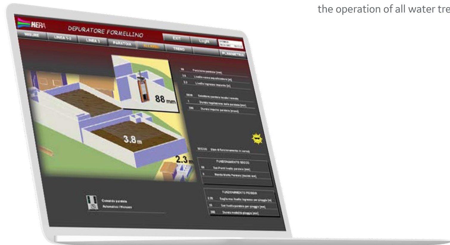
The water flow through the various stations of the water treatment plant is adjusted by controlling sluices.
