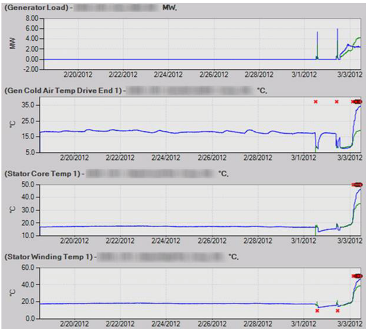
Screenshot increases in actual stator and cooling air temperatures (blue) versus expected values (green).
