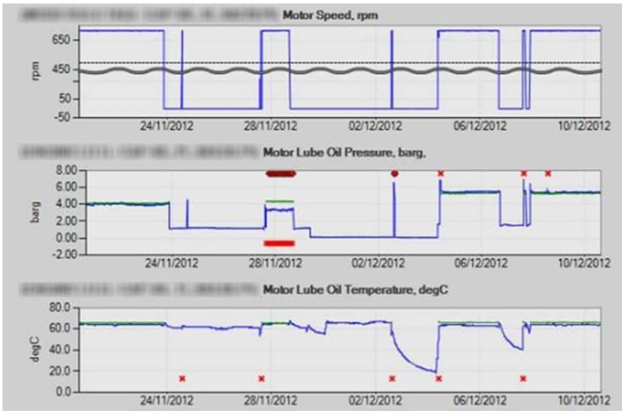
Screenshot depicting actual values (blue) and expected values (green). Lube oil pump motor speed shown in top graph. Lube oil pressure shown in middle graph. Lube oil temperature shown in bottom graph.
