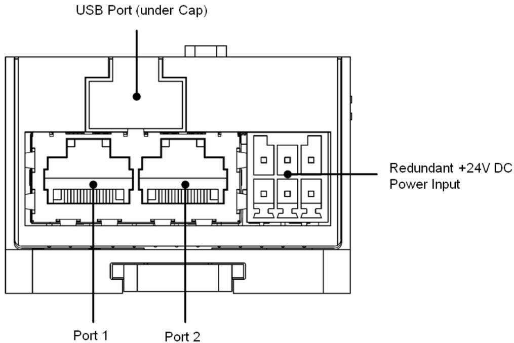
Devices connected to the RX3i CEP ports should have Ethernet Auto-negotiation enabled. The RX3i CEP Carriers and other participating devices can be connected in a daisy-chain/line, or star topology.
