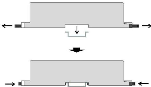
The carrier mounts on a standard EN 50022, 35mm x 7.5mm DIN rail. Conductive (unpainted) finish is required for proper grounding.
